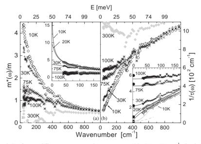
Fig. 1. (a)  $m^*(\omega)/m$  and (b)  $1/\tau(\omega)$  at different temperatures (insets: same quantities below  $200 \text{ cm}^{-1}$ ). Symbols: experimental data. Lines: calculation from the non-Drude fit. The inset of the right panel also shows  $\rho_{\text{DC}}\omega_P^2/(4\pi)$  (solid points) and the expected frequency dependence for heavy fermions (gray solid line) and for spin fluctuations (gray dashed line) at 10 K.
