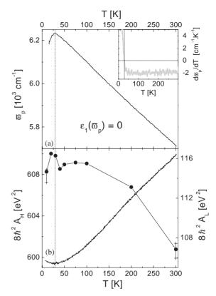
Fig. 2. (a) Plasma frequency and (b) spectral weight of  $\sigma(\omega)$  above and below 6000 cm<sup>-1</sup>.
