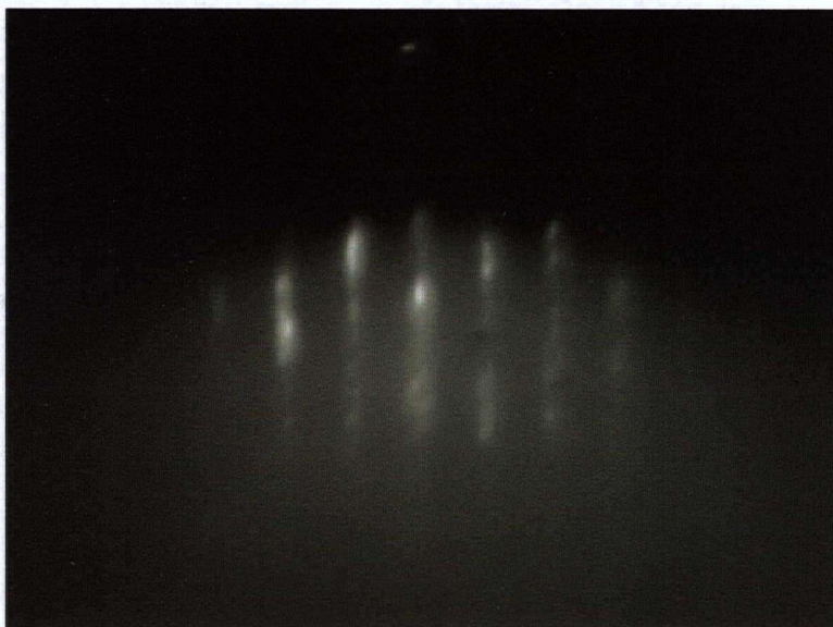
Figure 3.2: A RHEED diffraction pattern of a Mica sample. The 2-D nature of the diffraction pattern is evident in the extended, rod-like nature of the diffraction spots.
