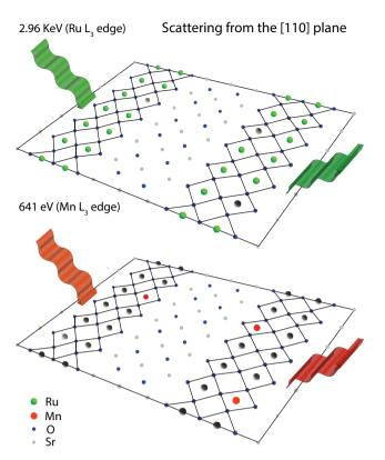
Figure 1 | Scattering from Sr<sub>3</sub>(Ru<sub>1-x</sub>Mn<sub>x</sub>)<sub>2</sub>O<sub>7</sub> along the [110] plane; one can see the Mn-substituted RuO<sub>2</sub> bilayers, separated by SrO planes. (a) When the x-ray energy is tuned to the Ru L<sub>3</sub> edge (2.96 KeV), the scattering signal is determined by the Ru atoms (green); (b) on the converse, at the Mn L<sub>3</sub> edge (641 eV), only the Mn atoms (red), occupying ~10% of the sites, contribute to the scattering signal.
