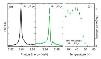
Figure 2 | Ru resonance REXS results from 10% Mn substituted Sr<sub>3</sub>(Ru<sub>1-x</sub>Mn<sub>x</sub>)<sub>2</sub>O<sub>7</sub> (x = 0.1). (a) Energy profile of the (1/4, 1/4, 0) peak across the Ru L<sub>2,3</sub> edge at T = 20 K. (b) Temperature dependence of the integrated intensity of the (1/4, 1/4, 0) peak at the Ru L<sub>2</sub> edge; the energy position (2968 eV) of the measurement is shown by the arrow in panel (a).
