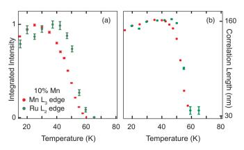
Figure 5 | Temperature dependence of the (a) normalized integrated intensity and (b) correlation length of the (1/4, 1/4, 0) superlattice order, measured at the Mn (red) and Ru (green) L-edges for 10% Mn-substitution.
