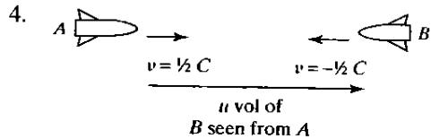
$$v_B = \frac{v_A + u}{1 + \frac{v_A u}{c^2}} \left\{ \begin{array}{l} -\frac{c}{2} = \frac{\frac{c}{2} + u}{1 + \frac{u \frac{c}{2}}{c^2}} \\ \text{Solve for } u \end{array} \right.$$
