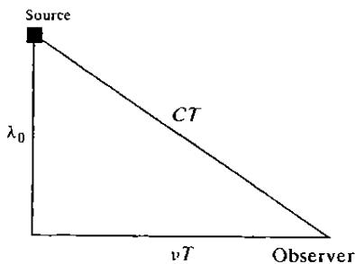
Take the distance from source to horizontal path of observer equal to the wavelength ( $\lambda_0$ ) emitted by source.  $T_0 = \frac{\lambda}{C}$  is period if observer were at rest.
