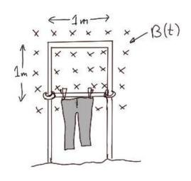
a) The increasing magnetic field gives an increasing flux through the square conducting loop.
