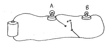
In the diagram shown, predict what will happen to the brightness of bulbs A and B when the switch is closed. Test your prediction with the simulator. Explain the results.
