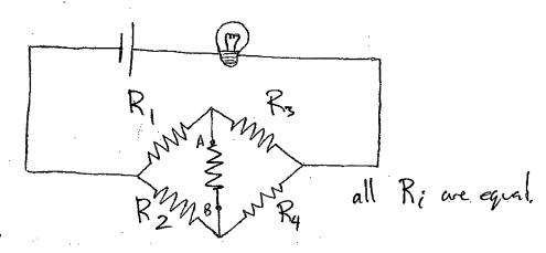
In the circuit shown above, a new resistor is added between points A and B. Does the light bulb get brighter, dimmer, or stay the same? Check your prediction. Explain the result.
