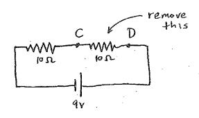
In the same circuit from problem 2 (shown schematically above) what is the potential difference between points C and D? Predict what the potential difference will be after you remove the indicated resistor. Use the simulator to check your result. Explain this result.
