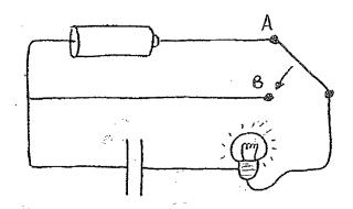
The circuit shown above includes a light bulb, a battery, and a capacitor. Predict what will happen when the switch is moved from A to B. Check your prediction using the real circuit components. Explain why the process you observe is not instantaneous, and explain how you could estimate the amount of time it takes based on the capacitance (how much charge there is on the capacitor for a given voltage) and the resistance of the bulb.
