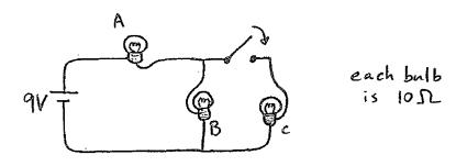
In the circuit shown, predict what will happen to the brightness of bulb A when the switch is closed. Test your prediction with the simulator. Explain the results.
