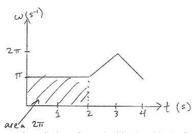
Question 8: The angular velocity  $\omega$  for a wheel is plotted in the figure above. Starting from time 0, how long is it before the wheel makes one complete rotation?
