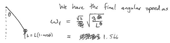
During the swing, the angular speed increases from 0 to this value. So we can say that the time is at least  $t_{min} = \frac{\frac{\pi}{2}}{\omega f} = 1.0035$
