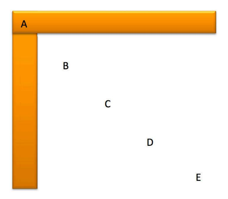
A crude boomerang is constructed by gluing two thin pieces of wood together as shown. Where is the center of mass?
