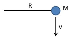
A ball of mass M revolves in a circular path on the end of a string. Using L = I  $\omega$ , calculate the angular momentum of the ball in terms of M, V, and R.
