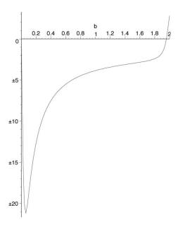
Figure D.3: The force between two loops displaced a distance b apart along a direction in their plane.
