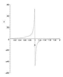
Figure D.2: The force between two loops on a common axis perpendicular to their planes as a function of the radius of one b changing with respect to the other a = 1.
