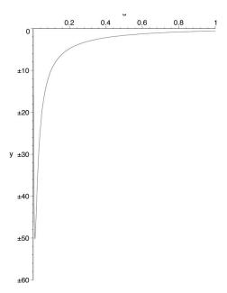
Figure D.1: The force between two current loops on a common axis perpendicular to their planes as a function of the distance d between them.
