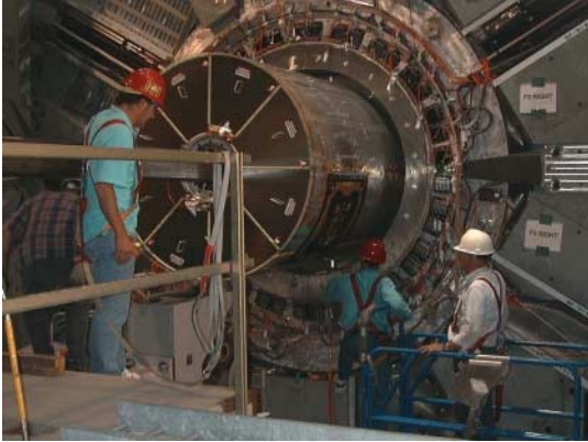
The drift chamber being integrated with the rest of the BaBar detector.
