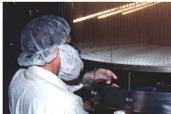
TRIUMF scientist Robert Henderson finalizes the construction of the BaBar drift chamber.
