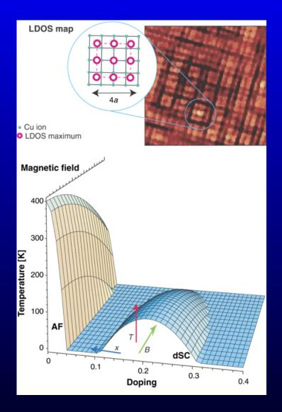
Checkerboard patterns in electron LDOS appear to be universal: encountered outside the superconducting dome in the underdoped region.
