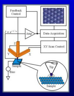
Scanning Tunneling Microscopy -images topography and local density of states
