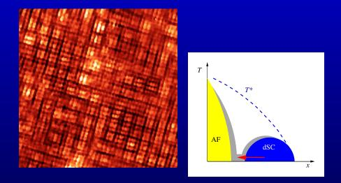
Scanning Tunneling Microscopy -images topography and local density of states Checkerboard pattern in LDOS of NaCCOC [Hanaguri *et. al*, Nature 2004]
