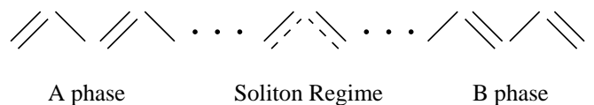
FIG. 7: A soliton excitation in polyacetylene. To the far "left" the chain is in the A phase of its ground state, and to the far "right" the chain is in the B phase of its ground state. The soliton is localized in the region in between these two phases.
