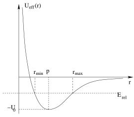
Fig 1. Effective potential for  $l \neq 0$ , and turning points for a value  $E_{rel} < 0$ .
