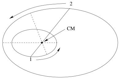
Fig 4. The motion of the two objects, when the CM (the focus of both ellipses) is at rest. If the CM is not at rest, just imagine moving the focus uniformly in some direction, as the masses rotate on ellipses about it. That's a bit too difficult for me to draw.
