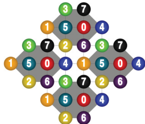
FIG. 7. (Color online) N = 32 cluster divided into eight groups labeled 0 = 7 . The spins within each group are connected by multiples of (2a, \pm 2a) . Spins from a particular group are always in the same environment, e.g., 1 always 4, 5, 6, and 7 as neighbors.
