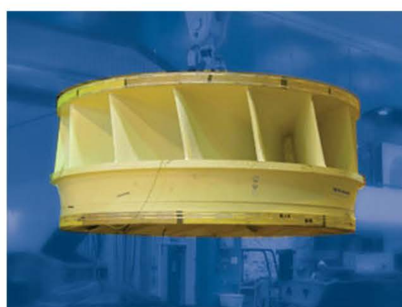
One of 10 turbines of the G.M. Shrum Generating Station
