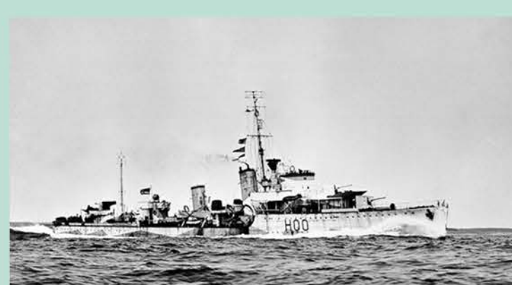
HMCS Restigouche, with Mann's high-resolution "286" radar at the masthead.
