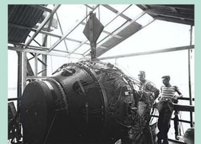
"The Gadget": the first nuclear bomb to be tested (July 1945), with Christy's "pit" at its core
