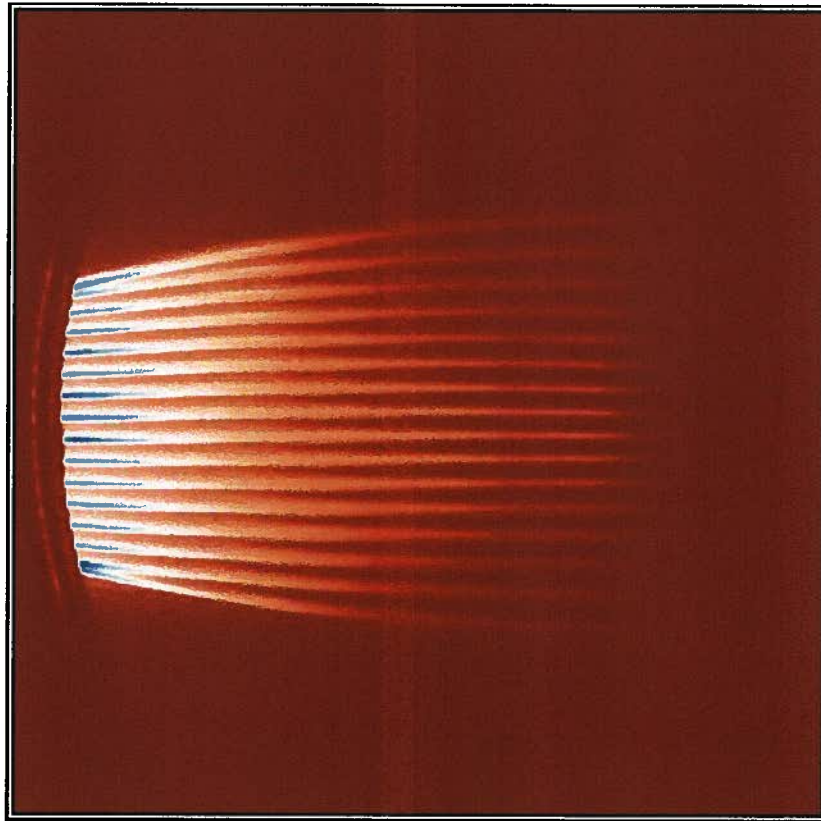
Figure 2.1. The raw data from a slit array calibration experiment. The left to right direction is parallel to the energy axis, while the up to down direction is roughly the angle axis. If the angular axis is straight, then the lines will be straight, so angle distortion is apparent in the curvature.
