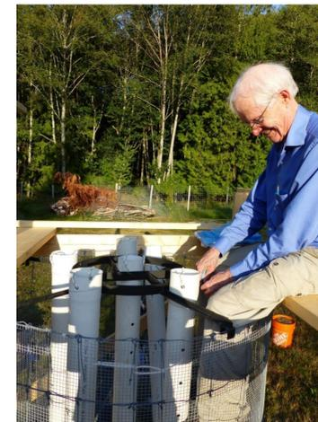
Attaching the PVC pipes to metal frame mounted on top of bioreactor cage. The pipes are pulled out 24 hr after loading, leaving behind 6 air channels to provide oxygen to the rapidly reproducing bacteria.
