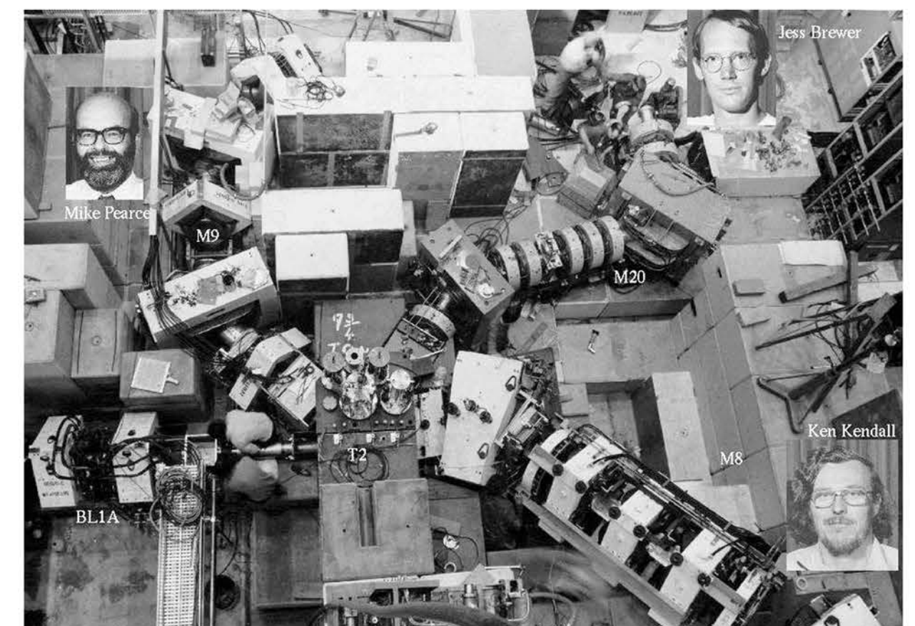
This photo shows a top view of the installation of the three beam channels that were originally installed on the T2 target at TRIUMF in the period 1973-74: M9 originally for studies of muonic and pionic atoms (inset: Mike Pearce, U. Victoria), the original M20 channel for \mu SR studies (inset: Jess Brewer, UBC & TRIUMF), and the “BioMed” channel M8 used for negative pion radiation therapy for cancer treatment (inset: Ken Kendall, with BC Cancer at the time). Photo provided by Jess Brewer.
