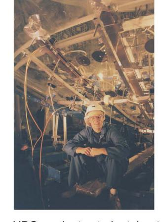
**UBC** graduate student Jaret Heise, in clean-room gear, building the 12 m diameter 35 tonne heavy water vessel, made from ultra-low radioactivity acrylic.
